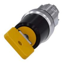
Key-operated switch O.M.R, 22 mm, round, metal, shiny, lock number 73033, yellow, with 2 keys, 2 switch positions O-I, latching, actuating angle 90°, 10:30h/13:30h, key removal I, Z=50-unit packaging
