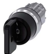
Key-operated switch O.M.R, 22 mm, round, metal, shiny, lock number 73034, black, with 2 keys, 3 switch positions I>O<II, momentary contact on the left, latching on the right, actuating angle  $2x45^{\circ}$ , 10:30h/12h/13:30h, Key removal II, with laser labeling, upper case and lower case, always upper case at the beginning of the word
