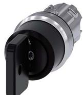
Key-operated switch O.M.R, 22 mm, round, metal, shiny, lock number 73034, black, with 2 keys, 3 switch positions I>O<II, momentary contact on the left, latching on the right, actuating angle 2x45°, 10:30h/12h/13:30h, Key removal II, with laser labeling, lower case
