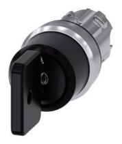
Key-operated switch O.M.R, 22 mm, round, metal, shiny, lock number 73034, black, with 2 keys, 3 switch positions I>O<II, momentary contact on the left, latching on the right, actuating angle  $2x45^{\circ}$ , 10:30h/12h/13:30h, Key removal II, with laser labeling, upper case
