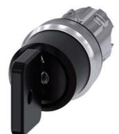
Key-operated switch O.M.R, 22 mm, round, metal, shiny, lock number 73034, black, with 2 keys, 3 switch positions I>O<II, momentary contact on the left, latching on the right, actuating angle  $2x45^{\circ}$ , 10:30h/12h/13:30h, Key removal II, with laser labeling, upper case and lower case, always upper case at beginning of line
