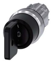
Key-operated switch O.M.R, 22 mm, round, metal, shiny, lock number 73034, black, with 2 keys, 3 switch positions I-O-II, latching, actuating angle  $2x45^{\circ}$ , 10:30h/12h/13:30h, Key removal I+O+II, with laser labeling, lower case
