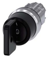
Key-operated switch O.M.R, 22 mm, round, metal, shiny, lock number 73034, black, with 2 keys, 3 switch positions I-O-II, latching, actuating angle  $2x45^{\circ}$ , 10:30h/12h/13:30h, Key removal I+O+II, with laser labeling, upper case
