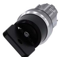
Key-operated switch O.M.R, 22 mm, round, metal, shiny, lock number 73034, black, with 2 keys, 2 switch positions O-I, latching, actuating angle 90°, 10:30h/13:30h, key removal I, with laser labeling, upper case
