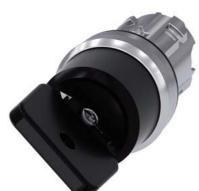
Key-operated switch O.M.R, 22 mm, round, metal, shiny, lock number 73034, black, with 2 keys, 2 switch positions O-I, latching, actuating angle 90°, 10:30h/13:30h, key removal O+I, with laser labeling, upper case and lower case, always upper case at the beginning of the word
