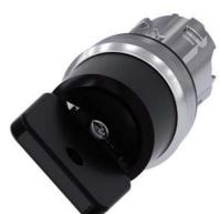
Key-operated switch O.M.R, 22 mm, round, metal, shiny, lock number 73034, black, with 2 keys, 2 switch positions O-I, latching, actuating angle 90°, 10:30h/13:30h, key removal O+I, with laser labeling, upper case
