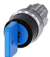
Key-operated switch O.M.R, 22 mm, round, metal, shiny, lock number 73038, blue, with 2 keys, 3 switch positions I-O-II, latching, actuating angle 2x45°, 10:30h/12h/13:30h, Key removal I+O+II, with laser labeling, upper case and lower case, always upper case at beginning of line
