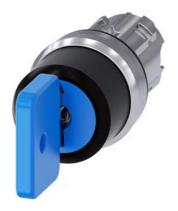
Key-operated switch O.M.R, 22 mm, round, metal, shiny, lock number 73038, blue, with 2 keys, 3 switch positions I-O-II, latching, actuating angle 2x45°, 10:30h/12h/13:30h, key removal O, with laser labeling, inscription or symbol Customer-specific selection with SIRIUS ACT configurator (CIN)
