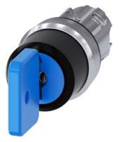
Key-operated switch O.M.R, 22 mm, round, metal, shiny, lock number 73038, blue, with 2 keys, 3 switch positions I-O-II, latching, actuating angle  $2x45^{\circ}$ , 10:30h/12h/13:30h, key removal O, with laser labeling, lower case
