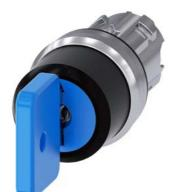
Key-operated switch O.M.R, 22 mm, round, metal, shiny, lock number 73038, blue, with 2 keys, 3 switch positions I-O-II, latching, actuating angle 2x45°, 10:30h/12h/13:30h, key removal O, with laser labeling, upper case
