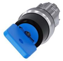
Key-operated switch O.M.R, 22 mm, round, metal, shiny, lock number 73038, blue, with 2 keys, 2 switch positions O-I, latching, actuating angle 90°, 10:30h/13:30h, key removal I, Z=50-unit packaging
