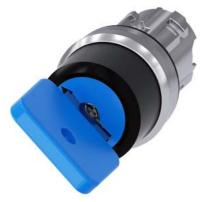
Key-operated switch O.M.R, 22 mm, round, metal, shiny, lock number 73038, blue, with 2 keys, 2 switch positions O-I, latching, actuating angle  $90^\circ$ , 10:30h/13:30h, key removal O+I, with laser labeling, lower case
