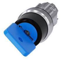
Key-operated switch O.M.R, 22 mm, round, metal, shiny, lock number 73038, blue, with 2 keys, 2 switch positions O-I, latching, actuating angle 90°, 10:30h/13:30h, key removal O+I, with laser labeling, upper case and lower case, always upper case at beginning of line
