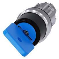
Key-operated switch O.M.R, 22 mm, round, metal, shiny, lock number 73038, blue, with 2 keys, 2 switch positions O<I, momentary contact type, Actuating angle 45°,  $10:30h/12h, \, key \, removal \, O, \, Z=50-unit \, packaging$
