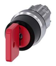
Key-operated switch O.M.R, 22 mm, round, metal, shiny, lock number 73037, red, with 2 keys, 3 switch positions I-O-II, latching, actuating angle 2x45°, 10:30h/12h/13:30h, Key removal I+O+II, with laser labeling, upper case and lower case, always upper case at the beginning of the word
