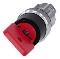
Key-operated switch O.M.R, 22 mm, round, metal, shiny, lock number 73037, red, with 2 keys, 2 switch positions O<I, momentary contact type, Actuating angle 45°, 10:30h/12h, key removal O, with laser labeling, inscription or symbol Customer-specific selection with SIRIUS ACT configurator (CIN)
