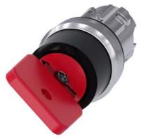
Key-operated switch O.M.R, 22 mm, round, metal, shiny, lock number 73037, red, with 2 keys, 2 switch positions O<I, momentary contact type, Actuating angle  $45^\circ$ , 10:30h/12h, key removal O, with laser labeling, upper case and lower case, always upper case at the beginning of the word
