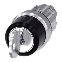
RONIS key-operated switch, 22 mm, round, metal, shiny, Lock No. 421, with 2 keys, 3 switch positions I-O-II, latching, actuating angle 2x45°, 10:30h/12h/13:30h, Key removal I+O+II, with laser labeling, lower case
