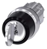
RONIS key-operated switch, 22 mm, round, metal, shiny, lock number 455, with 2 keys, 3 switch positions I>O<II, momentary contact type, actuating angle 2x45°, 10:30h/12h/13:30h, key removal O, with laser labeling, upper case and lower case, always upper case at beginning of line
