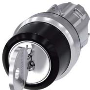
RONIS key-operated switch, 22 mm, round, metal, shiny, lock number 455, with 2 keys, 3 switch positions I-O-II, latching, actuating angle 2x45°, 10:30h/12h/13:30h, Key removal I+O+II, with laser labeling, upper case and lower case, always upper case at the beginning of the word
