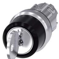
RONIS key-operated switch, 22 mm, round, metal, shiny, lock number 455, with 2 keys, 3 switch positions I-O-II, latching, actuating angle  $2x45^{\circ}$ , 10:30h/12h/13:30h, Key removal I+O+II, with laser labeling, lower case
