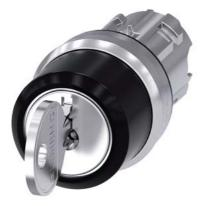
RONIS key-operated switch, 22 mm, round, metal, shiny, lock number 455, with 2 keys, 3 switch positions I-O-II, latching, actuating angle 2x45°, 10:30h/12h/13:30h, key removal O, with laser labeling, upper case and lower case, always upper case at the beginning of the word
