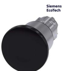
Mushroom pushbutton, 22 mm, round, metal, shiny, black, 40 mm, 3 switch positions, latches after pushing in, unlatches by pull-to-unlatch mechanism to center position, after pulling out the button Retraction to center position
