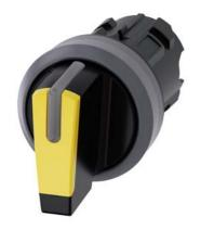
Selector switch, illuminable, 22 mm, round, plastic with metal front ring, yellow, selector switch, short, 3 switch positions I-O<II, left latching, right momentary contact type, actuating angle  $2x45^{\circ}$ , 10:30h/12h/13:30h
