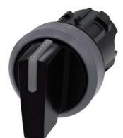
Illuminable selector switch, 22 mm, round, plastic with metal front ring, black, Selector switch short, 3 switch positions I-O<II, left latching, momentary contact type on the right, actuating angle  $2x45^{\circ}$ , 10:30 /12 /13:30, Z=50-unit packaging
