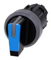
Selector switch, illuminable, 22 mm, round, plastic with metal front ring, blue, selector switch, short, 3 switch positions I>O<II, momentary contact type, actuating angle  $2x45^{\circ}$ , 10:30h/12h/13:30h, with laser labeling, inscription or symbol Customer-specific selection with SIRIUS ACT configurator (CIN)
