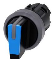
Selector switch, illuminable, 22 mm, round, plastic with metal front ring, blue, selector switch, short, 3 switch positions I>O<II, momentary contact type, actuating angle 2x45°, 10:30h/12h/13:30h, with laser labeling, lower case
