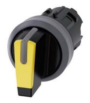
Selector switch, illuminable, 22 mm, round, plastic with metal front ring, yellow, selector switch, short, 3 switch positions I-O-II, latching, actuating angle  $2x45^\circ$ , 10:30h/12h/13:30h
