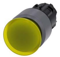
Illuminated mushroom pushbutton, 22 mm, round, plastic with metal front ring, yellow, 30 mm, latching, Pull-to-unlatch mechanism
