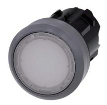
Illuminated pushbutton, 22 mm, round, plastic with metal front ring, white, pushbutton, flat, latching, Push-to-release mechanism, with laser labeling, inscription or symbol Customer-specific selection with SIRIUS ACT configurator (CIN)
