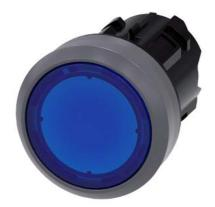
Illuminated pushbutton, 22 mm, round, plastic with metal front ring, blue, pushbutton, flat, latching, Push-to-release mechanism, with laser labeling, symbol number according to, ISO 7000 or IEC 60417
