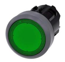
Illuminated pushbutton, 22 mm, round, plastic with metal front ring, green, pushbutton, flat, latching, Push-to-release mechanism, with laser labeling, symbol number according to, ISO 7000 or IEC 60417
