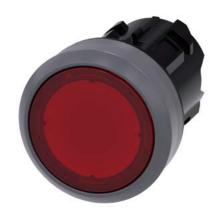
Illuminated pushbutton, 22 mm, round, plastic with metal front ring, red, pushbutton, flat, latching, Push-to-release mechanism, with laser labeling, lower case
