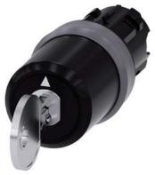
key-operated switch Siemens, 22 mm, round, plastic with metal front ring, lock number SSG10, with 2 keys, 3 switch positions I>O<II, momentary contact on the left, latching on the right, actuating angle  $2x45^\circ$ , 10:30h/12h/13:30h, key removal II
