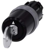
key-operated switch Siemens, 22 mm, round, plastic with metal front ring, lock number SSG10, with 2 keys, 3 switch positions I>O<II, momentary contact on the left, latching on the right, actuating angle  $2x45^\circ$ , 10:30h/12h/13:30h, key removal O
