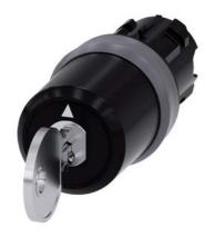
key-operated switch Siemens, 22 mm, round, plastic with metal front ring, lock number SSG10, with 2 keys, 3 switch positions I>O<II, momentary contact on the left, latching on the right, actuating angle 2x45°, 10:30h/12h/13:30h, key removal O, with laser labeling, inscription or symbol customer-specific selection with SIRIUS ACT configurator (CIN)
