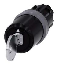
key-operated switch Siemens, 22 mm, round, plastic with metal front ring, lock number SSG10, with 2 keys, 3 switch positions I>O<II, momentary contact on the left, latching on the right, actuating angle 2x45°, 10:30h/12h/13:30h, key removal O, with laser labeling, upper case and lower case, always upper case at the beginning of the word
