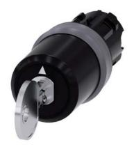
key-operated switch Siemens, 22 mm, round, plastic with metal front ring, lock number SSG10, with 2 keys, 3 switch positions I>O<II, momentary contact on the left, latching on the right, actuating angle  $2x45^{\circ}$ , 10:30h/12h/13:30h, key removal O, with laser labeling, lower case
