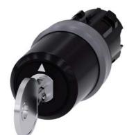
key-operated switch Siemens, 22 mm, round, plastic with metal front ring, special lock, with 2 keys, 3 switch positions I>O<II, momentary contact on the left, latching on the right, actuating angle  $2x45^{\circ}$ , 10:30h/12h/13:30h, key removal O
