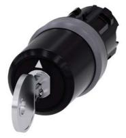
key-operated switch Siemens, 22 mm, round, plastic with metal front ring, lock number SSG10, with 2 keys, 3 switch positions I-O<II, left latching, momentary contact type on the right, actuating angle  $2x45^\circ$ , 10:30h/12h/13:30h, key removal O+I, with laser labeling, upper case and lower case, always upper case at beginning of line
