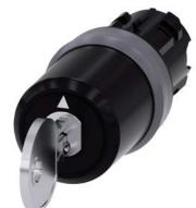
key-operated switch Siemens, 22 mm, round, plastic with metal front ring, lock number SSG10, with 2 keys, 3 switch positions I-O<II, left latching, momentary contact type on the right, actuating angle  $2x45^{\circ}$ , 10:30h/12h/13:30h, key removal I, with laser labeling, lower case
