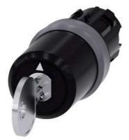
key-operated switch Siemens, 22 mm, round, plastic with metal front ring, special lock, with 2 keys, 3 switch positions I-O<II, left latching, momentary contact type on the right, actuating angle  $2x45^{\circ}$ , 10:30h/12h/13:30h, key removal I
