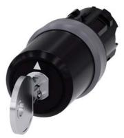
key-operated switch Siemens, 22 mm, round, plastic with metal front ring, special lock, with 2 keys, 3 switch positions I-O-II, latching, actuating angle 2x45°, 10:30h/12h/13:30h, key removal I+O+II
