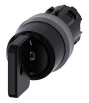
Key-operated switch O.M.R, 22 mm, round, plastic with metal front ring, lock number 73034, black, with 2 keys, 3 switch positions I-O-II, latching, actuating angle  $2x45^{\circ}$ , 10:30h/12h/13:30h, Key removal I+O+II
