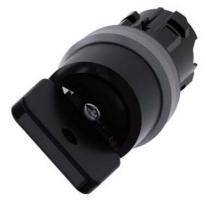
Key-operated switch O.M.R, 22 mm, round, plastic with metal front ring, lock number 73034, black, with 2 keys, 2 switch positions O-I, latching, actuating angle 90°, 10:30h/13:30h, key removal O, Z=50-unit packaging
