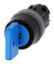
Key-operated switch O.M.R, 22 mm, round, plastic with metal front ring, lock number 73038, blue, with 2 keys, 3 switch positions I-O-II, latching, actuating angle 2x45°, 10:30h/12h/13:30h, Key removal I+O+II, with laser labeling, upper case and lower case, always upper case at the beginning of the word
